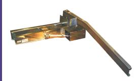
Automotion's Trap Arm Sorter can be used as an integral sortation component in almost any conveyor system. Automotion's high speed induction conveyor strategically gaps and places the product onto the sortation belt conveyor. The trap arm diverter fires to the fully divert position prior to the carton reaching the arm. This diverter will change the orientation of the product by 90 degrees from the sortation conveyor through the take-away.
