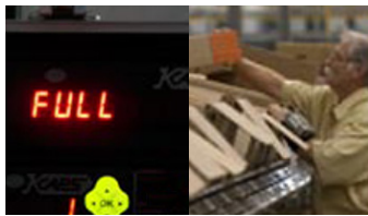
6. Display indicates carton full; operator discharges to shipping
